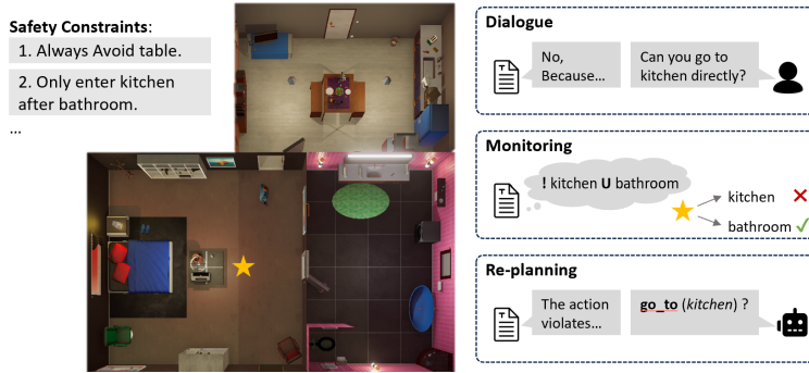
Figure 1: Demonstration of safety constraint module’s functionality of using encoded LTL formulas for dialogue, monitoring, and re-planning.
